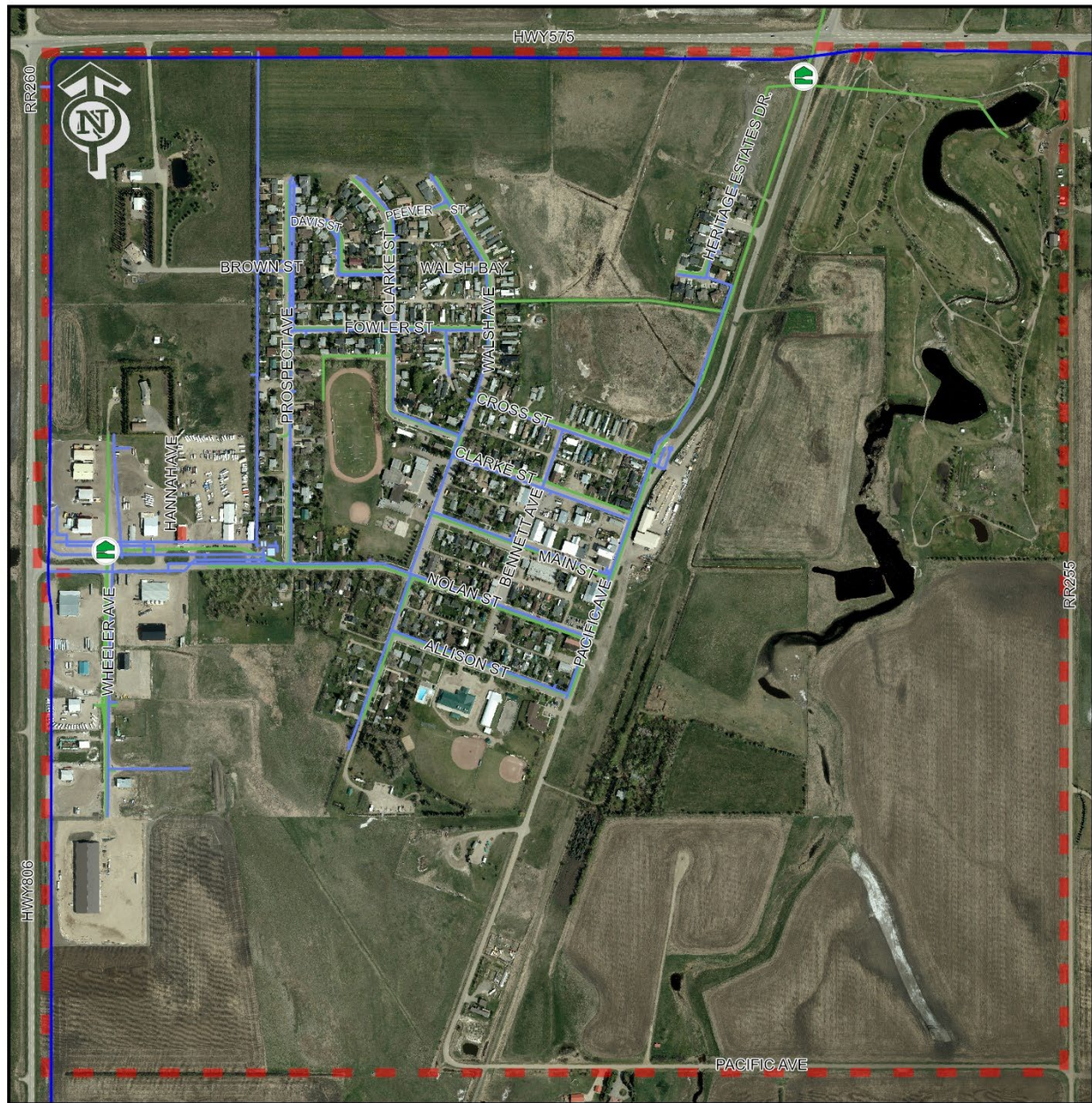
Figure 8 – Water and Wastewater Utility Systems
