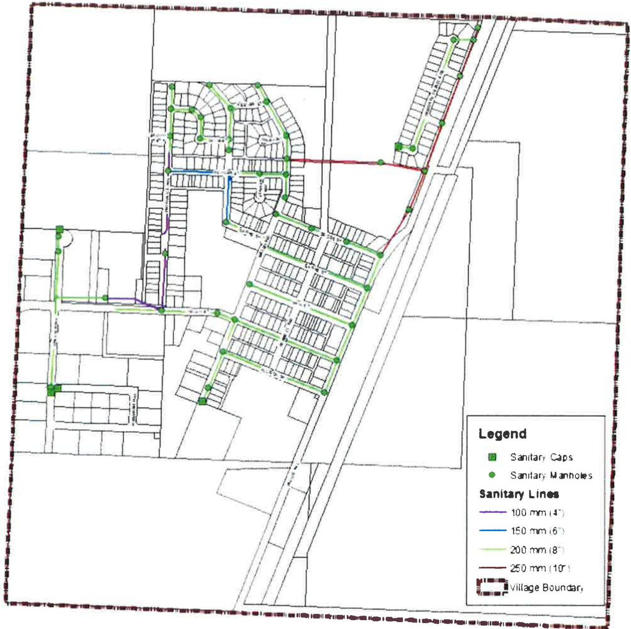
Figure 5: Waste Water System (Sanitary Sewer)
